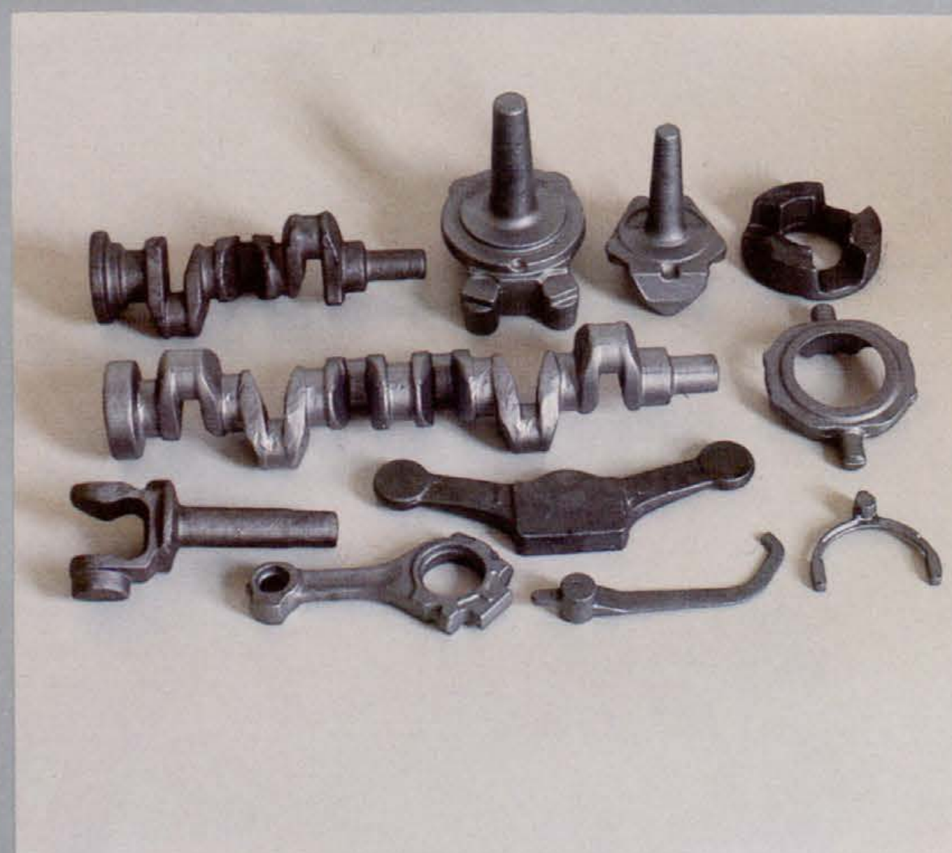
DROP FORGINGS Weight from 2 to about 100 kg Manufacturer: TAM Maribor
