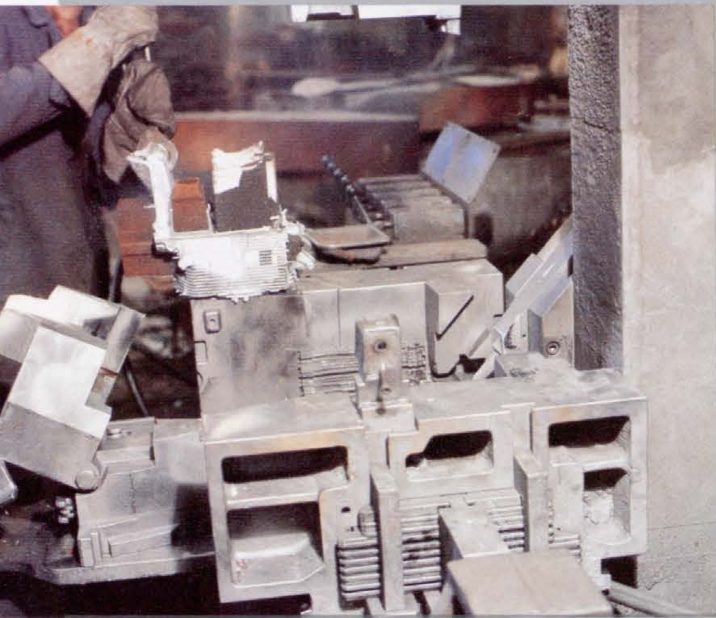
MOULDS for Al-alloys Casting Manufacturer: TAM Maribor
