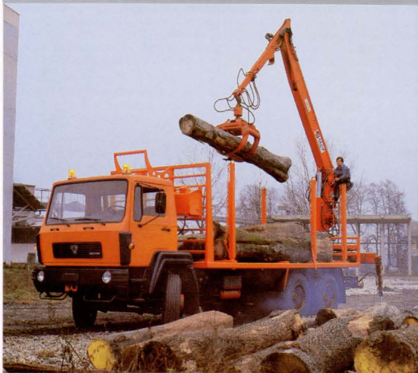
Timber Transport Vehicle TAM 260 T26 B-GO 6 × 4
