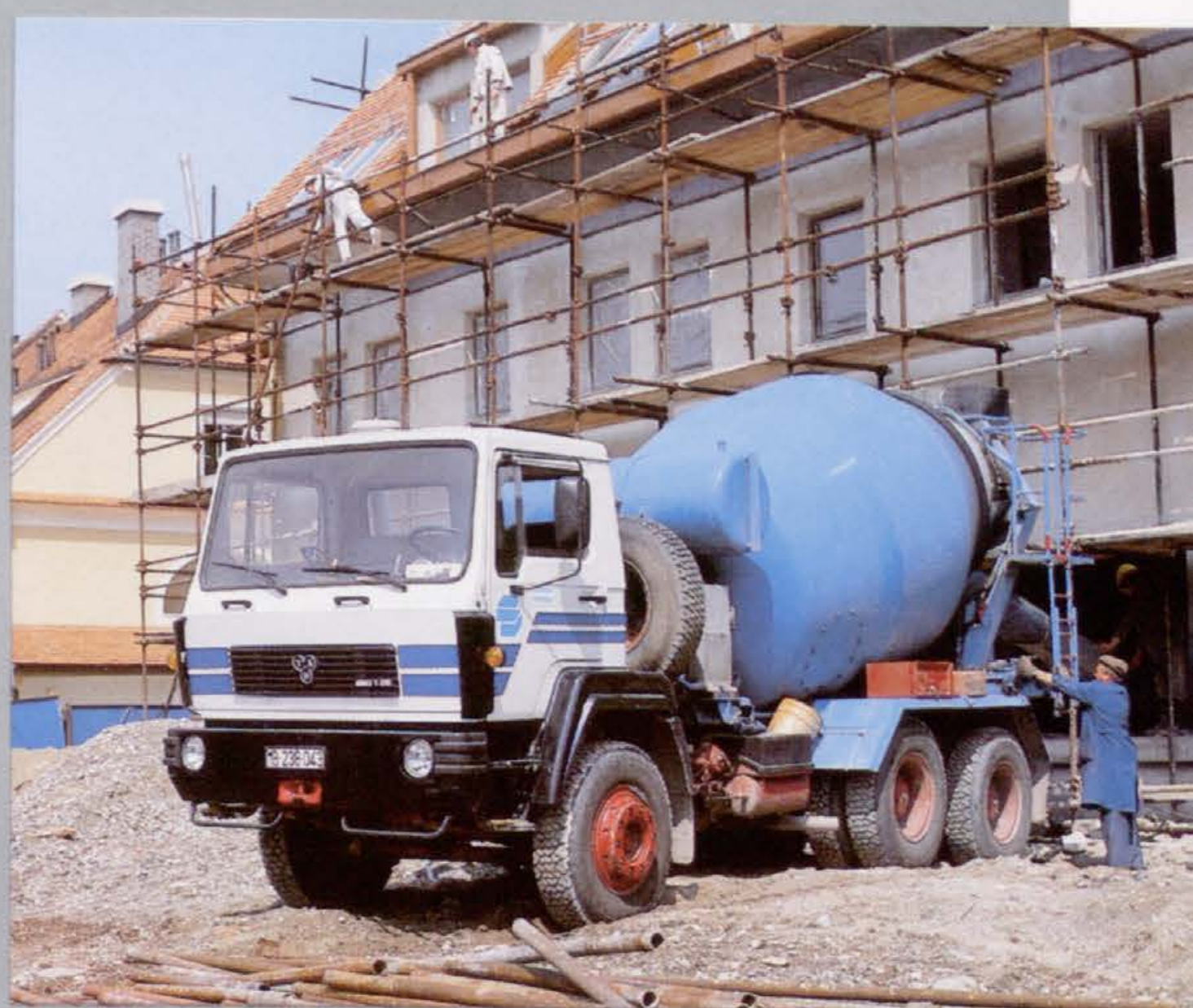
Concrete Mixer TAM 260 T26 B-BM 6 × 4
